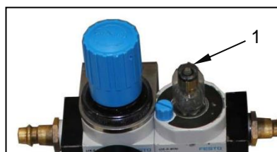
Fig. 5-2 Filling the service unit
