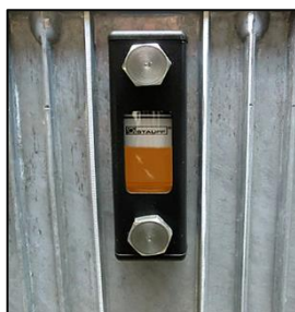
Fig. 8-1 Optimum oil level
