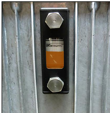
Fig. 5-1 Optimum oil fill level
