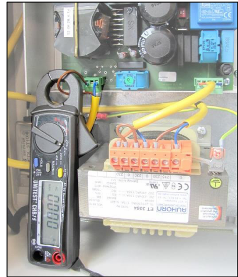
Fig. 8-4 Stunning current strength measurement
