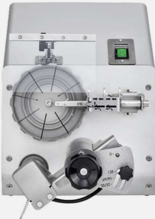
*Figure: Standard variant with steeling device for blades Ø 69 -128mm
